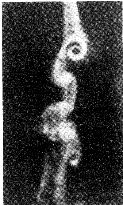
Fig. 5 Counter-rotating vortex pairs generated near the impinging plane.
